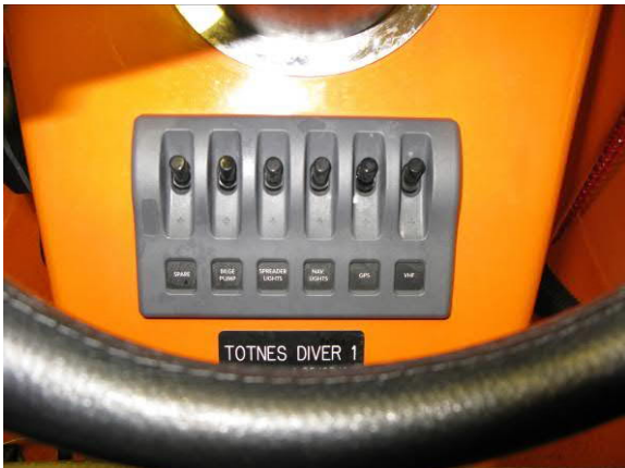
Both boats have a switch panel beneath the steering wheel (the picture shows TD1). All switches should be in the off (up) position when the boat is not in use.
