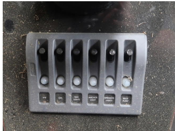
The switches are clearly labelled and those for the chartplotter and radio need to be turned on before use. It is essential that the units are turned on and off using their individual power buttons and not by using the switch panel.
