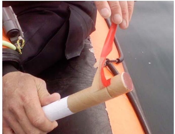
This short length of tube is the striker, which has an edge "just like the side of a box of matches". You will see on the end of the longer tube of the Thunderflash what looks like a fat match. Gently strike the fat match across the red area of the short length of tube (i.e. the striker). **You now only have 5-7 seconds before it goes off, so get rid of the Thunderflash immediately, throwing it away from the boat, and wait for the bang!**
