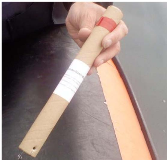
In order for the divers to hear the Thunderflash it needs to be weighted, and fishing weights are provided for this purpose, which are attached to the base of the tube with a paper clip!
